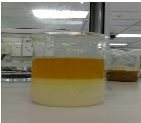
Figure 3.6: Biodiesel after 1 hour washed with hot water
