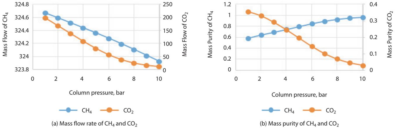
Figure 4 Effects of column pressure
