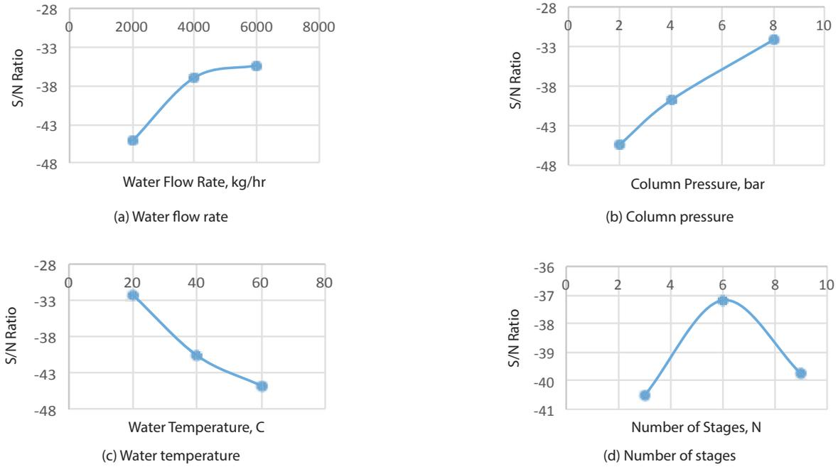
Figure 7 S/N ratio v/s factor level
