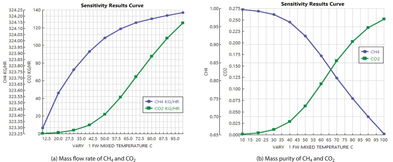
Figure 5 Effects of water temperature
