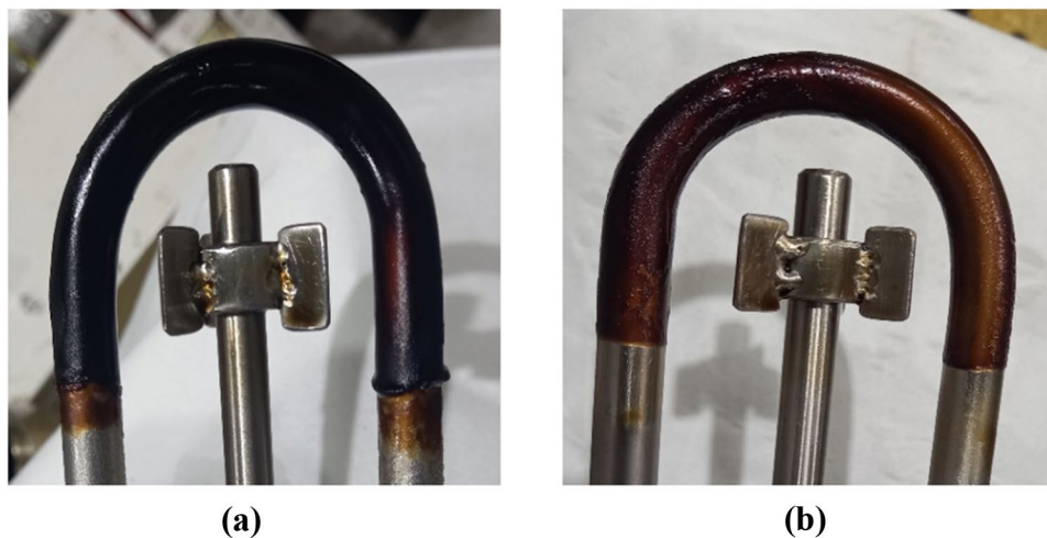
Fig. 4 Cold finger temperature effect on the deposition of wax, a 5 °C and b 10 °C
