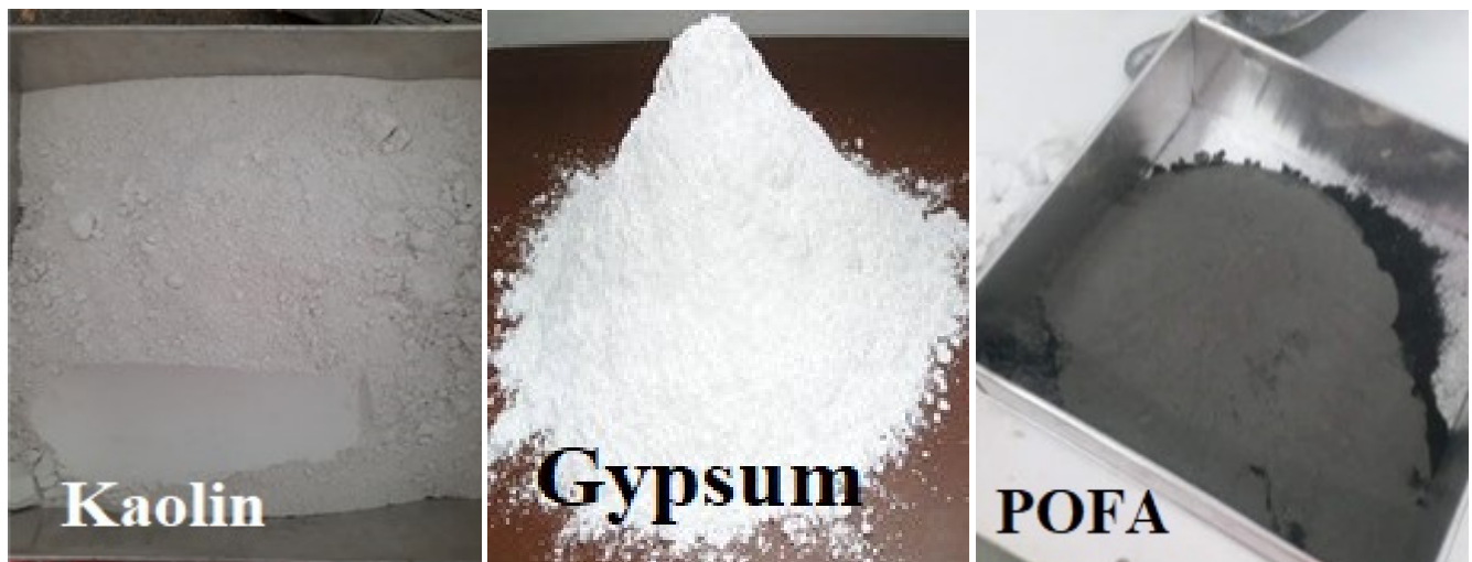
Figure 2. Used POFA, kaolin, gypsum in experimental laboratory work.
