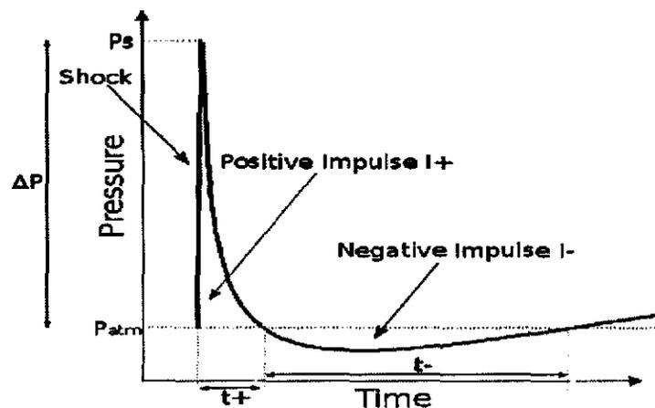
Figure 2.2 Typical ideal free-air blast wave pressure-time graph
