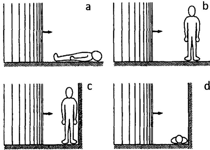
Figure 2.6 Position of human body. (a) No obstruction of incident wave:  $P = P_s$ .
