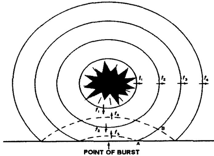
Figure 2.4 Blast wave from a surface burst
