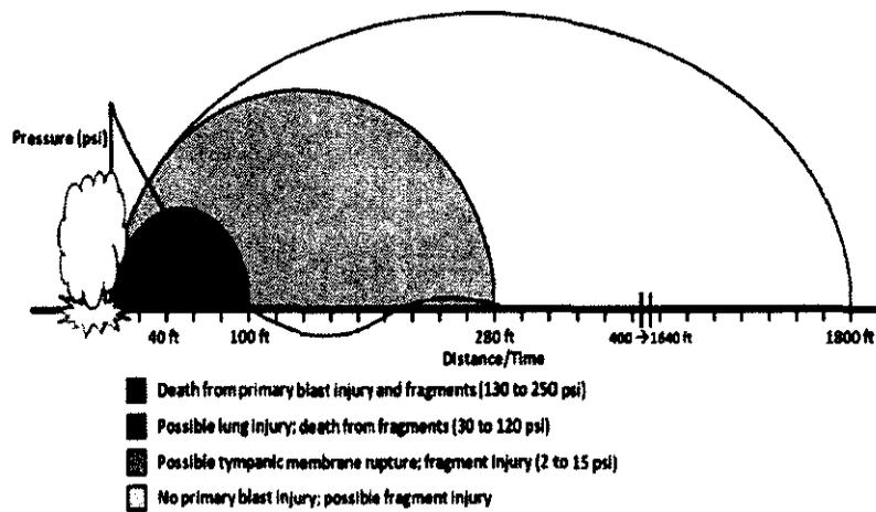
Figure 2.5 Illustration of Friedlander curve with maximum effective radius of primary and secondary blast injuries of an open spaced without any barrier wall, 155 mm mortar shell explosion with 200 lbs (100 kg) of TNT equivalent
