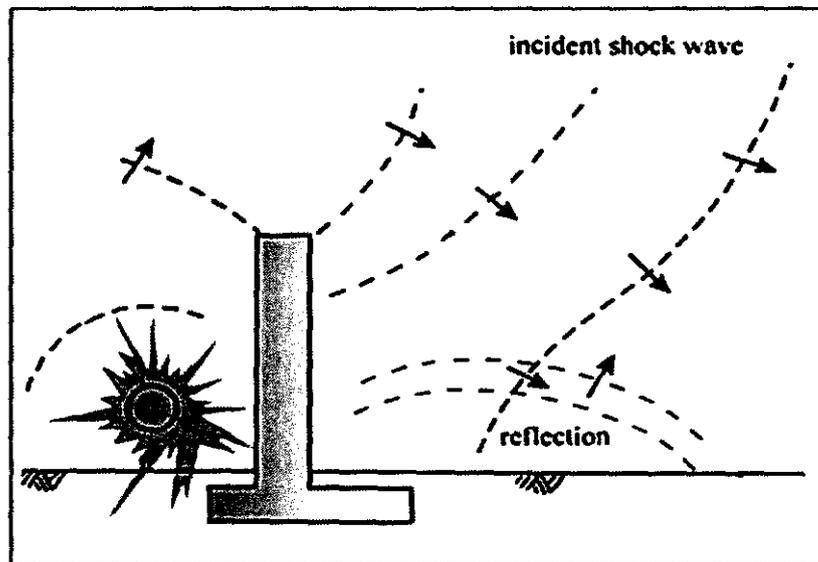
Figure 2.8 Blast wave diffraction over a barrier wall.
