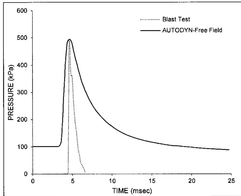
Figure 4.1 Peak blast pressure between numerical simulation and actual blast test.
