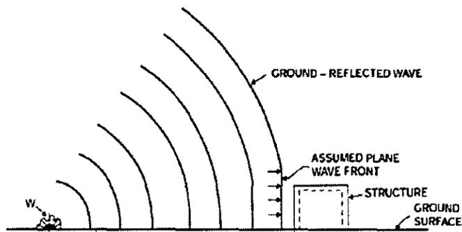
Figure 2.1 Illustration of Blast Wave Propagation
