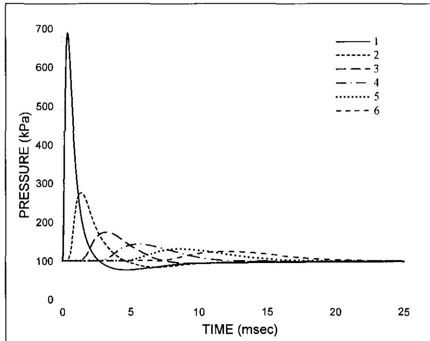
Figure 4.2 Pressure profile without RC wall
