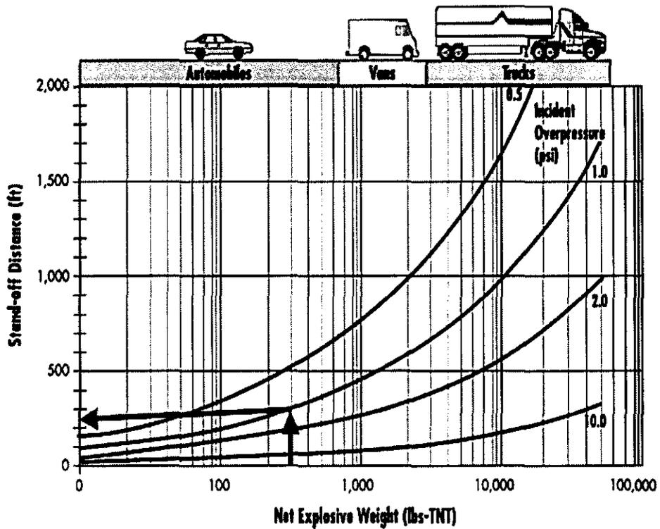
Figure 2.7 Chart of blast pressure against stand-off distance
