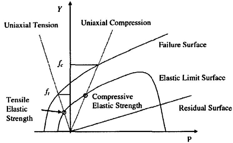
Figure 2.10 Maximum strength, yield strength and residual strength surfaces.
