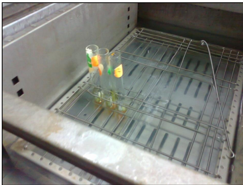
Figure 3.9: The samples were heated in water bath at 90°C -100°C
