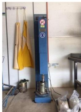
**Figure 2.** Automatic soil compactor used to crush soil samples
