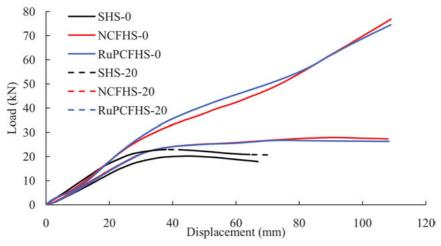
Fig. 5. Load-deflection curves of columns under lateral load
