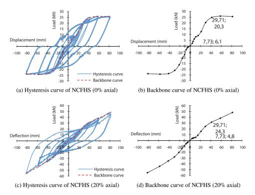
Fig. 7. Hysteresis and backbone curve of NCFHS
