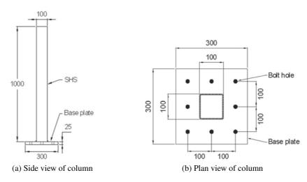
Fig. 1. Schematic drawing of column specimens
