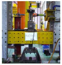
(b) Test setup with axial load
