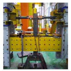
(a) Test setup without axial load
