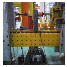
(a) Test setup without axial load
