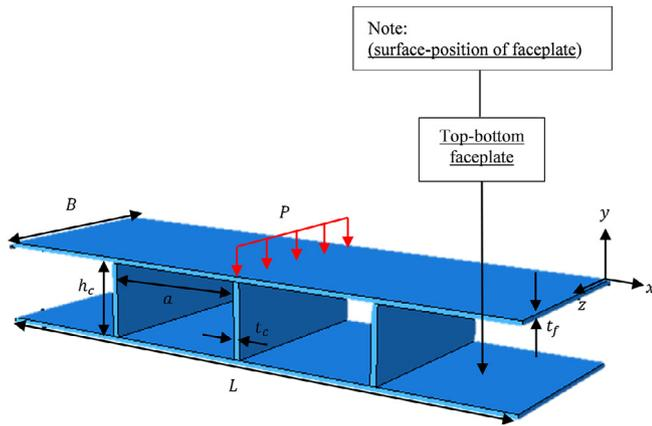
Fig. 2. The structure of I-core sandwich steel plate.
