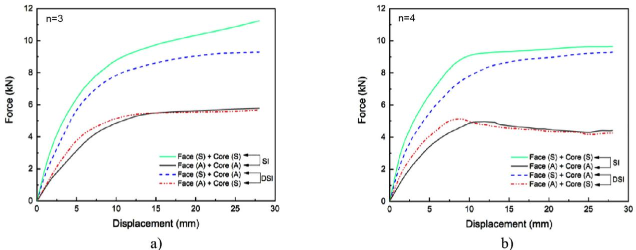
Fig. 9. Result for SI and DSI material on or either element of I-core Sandwich plate: a) n: 3, and b) n: 4.
