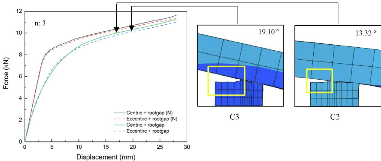
Fig. 11. Failure of weld position at n:3 T-joint: centric + rootgap (C2), and eccentric + rootgap (C3).
