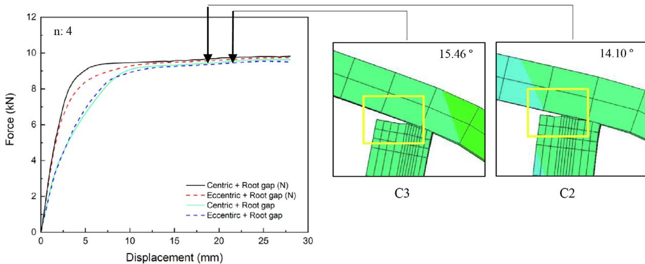
Fig. 12. Failure of weld position at n:4 T-joint: centric + rootgap (C2), and eccentric + rootgap (C3).
