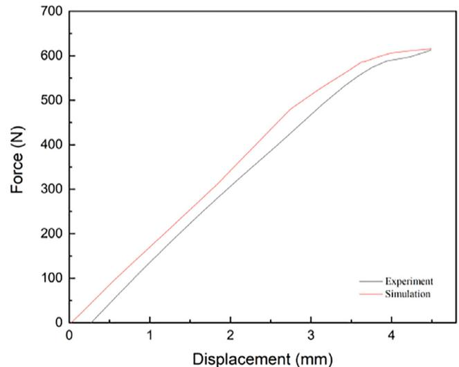
Fig. 5. Experiment and simulation comparison for laser-welded I-core galvanize steel sandwich plate.
