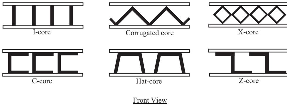
Fig. 1. Different topologies of sandwich plate.
