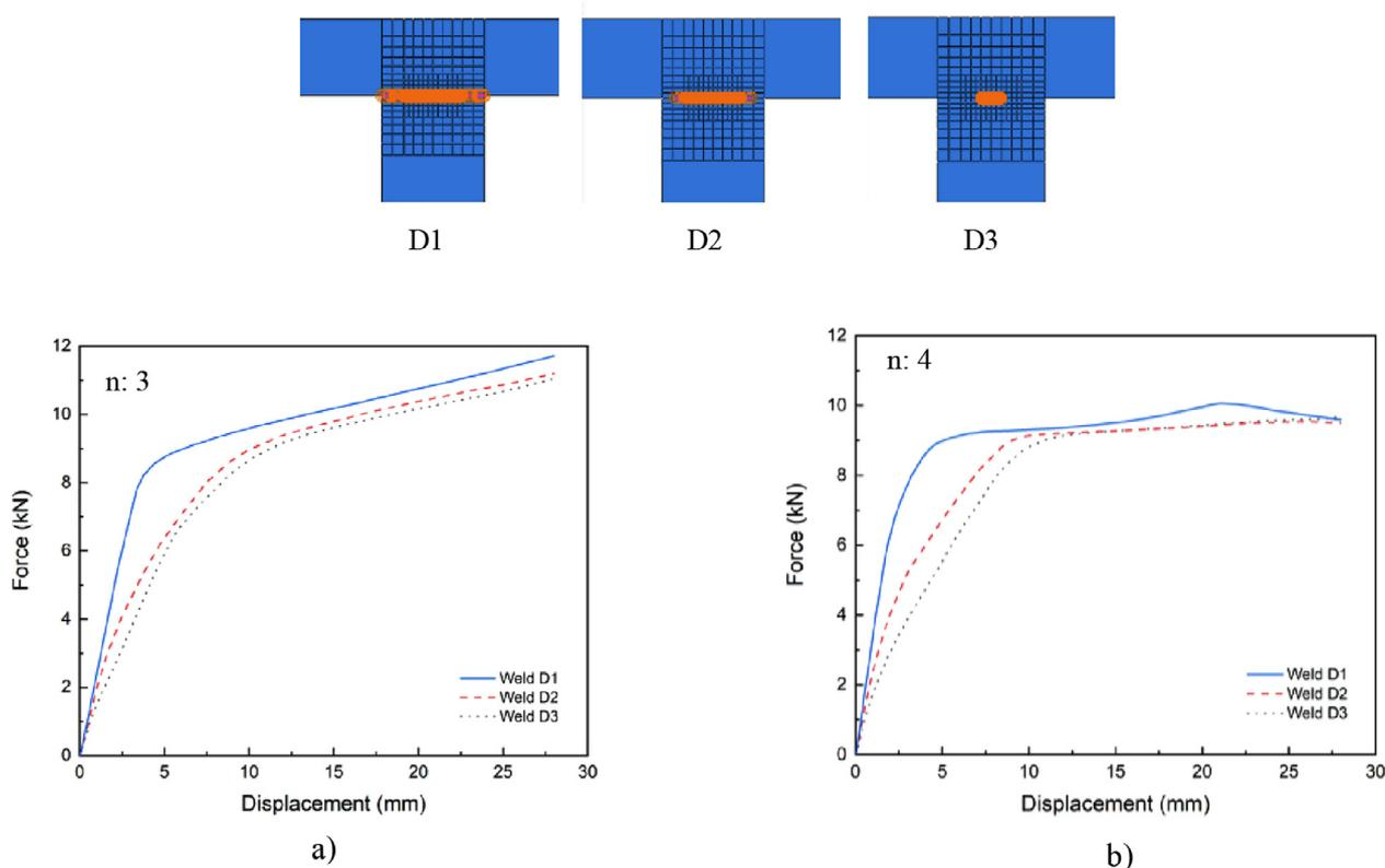
Fig. 13. Weld width comparison of different length D1, D2, and D3 for n: 3 and n: 4.
