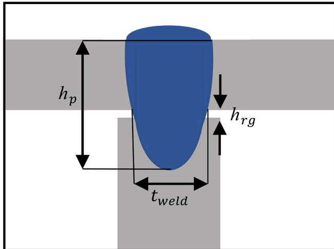
Fig. 4. Illustration of laser weld geometry parameter.
