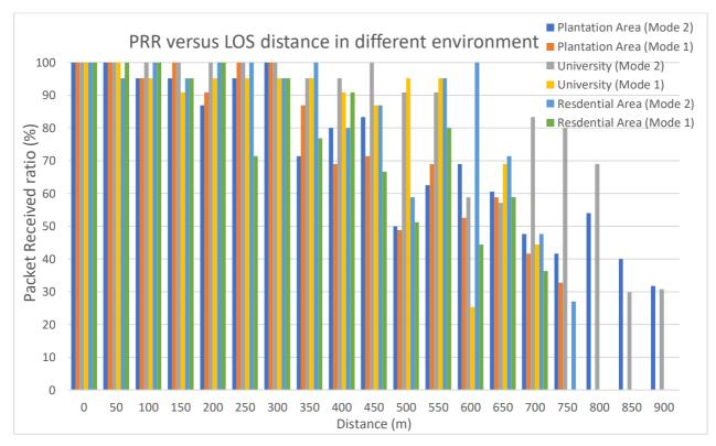
Figure 10. The graph for PRR versus LOS distance sensors in different environments
