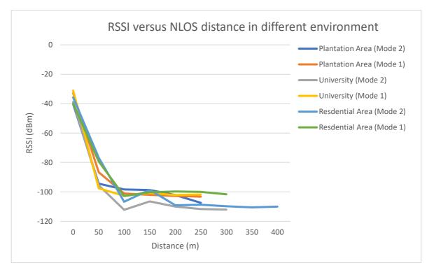
Figure 11. The graph for RSSI versus NLOS distance sensors in different environments
