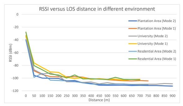
Figure 9. The graph for RSSI versus LOS distance sensors in different environments
