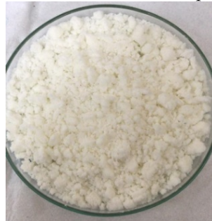
Figure 3. Microcapsules of polyurea-formaldehyde (PUF) with linseed oil as a corrosion inhibitor agent, stirred at a stirring rate of 300 rpm.
