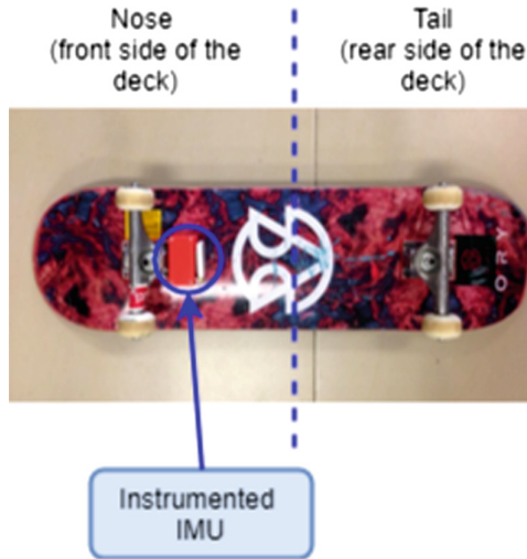
Fig. 2. The attachment of the instrumented IMU on the deck
