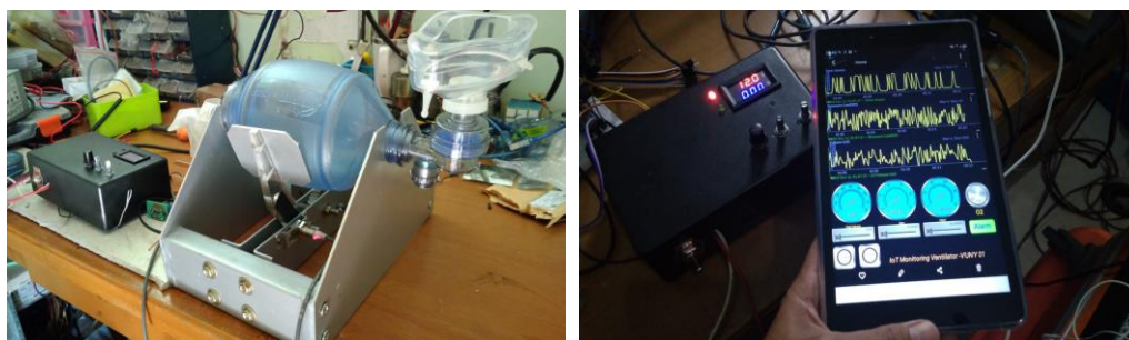
Figure 6. Prototype of Ventilator Monitoring System
