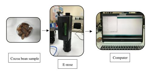
Figure 2. Flow of Collecting Odor of Cocoa Bean Sample
