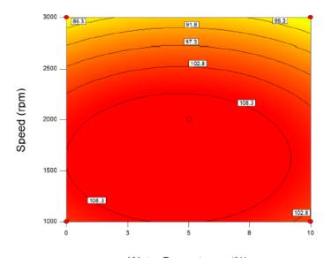
Water Percentages (%) **Fig. 3.** Interactive contour plot for engine torque at difference percentages of water and speed
