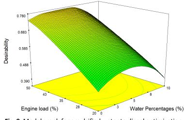
Fig. 9. Model graph for emulsified water to diesel optimization
