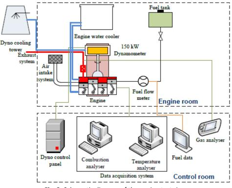
Fig. 2. Schematic diagram of the engine test rig
