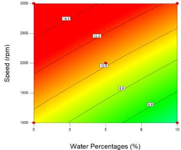
**Fig. 8.** Interactive contour plot for CO<sub>2</sub> at difference percentages of water and speed
