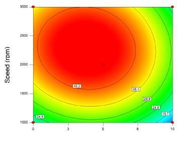
Water Percentages (%) Fig. 4. Interactive contour plot for BTE at difference percentages of water and speed
