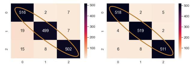
Figure 18. Confusion matrix of NEEEMD and NEEEMD + DCGAN at the turning point for blade fault diagnosis.
