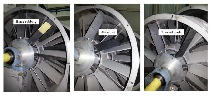
Figure 5. Different blade fault conditions.
