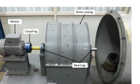
Figure 4. Test rig to simulate blade fault.
