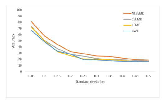
Figure 15. Performance of blade fault localization classifier on noisy data.
