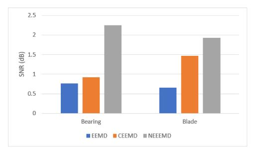
Figure 7. SNR values for reconstructed signals of bearing and blade samples.
