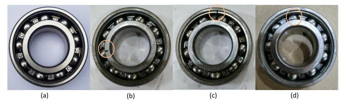
Figure 3. Four bearing conditions (a) normal condition, (b) inner race fault, (c) outer race fault, (d) ball fault.
