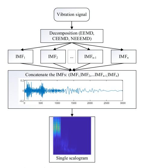
Figure 10. The process of scalogram generation.
