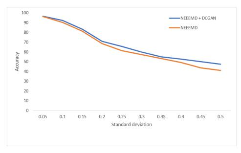
Figure 20. Performance of bearing fault classifier on noisy data.
