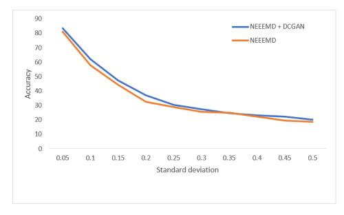
Figure 22. Performance of blade fault localization classifier on noisy data.
