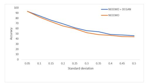
Figure 21. Performance of blade fault diagnosis classifier on noisy data.
