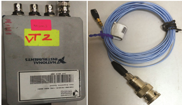
Fig. 2 — NI acoustic and vibration data logger and cable uni-axial
