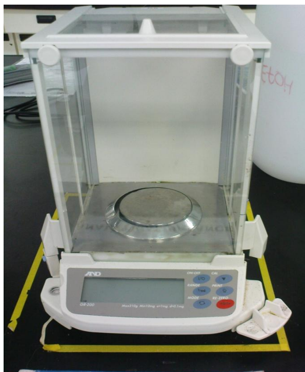
Figure A.8: Analytical balance to weight dye and DWH
