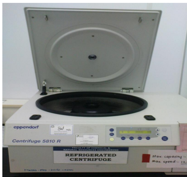
Figure A.7: Refrigerated centrifuge to separate the supernatant
