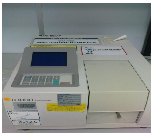
Figure A.6: UV-Vis Spectrophotometer for analysis of sample
