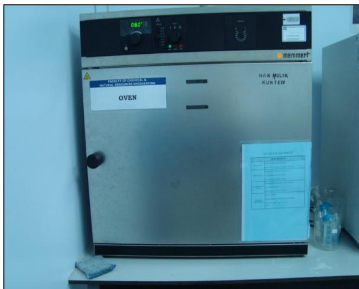
Figure A.5: Oven to dry the water hyacinth
