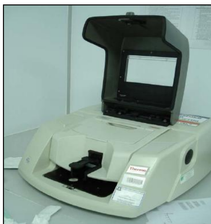
Figure A.2: Fourier Transform Infra Red (FT-IR) to determine the functional group of water hyacinth
