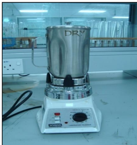
Figure A.1: Blender to blend water hyacinth to a smaller particle
