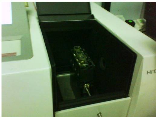
Figure 17: Sample reading via UV-VIS spectrophotometer
