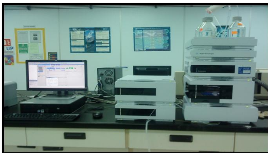
Figure 2.12 : High Performance Liquid Chromatography (HPLC) that using SUPELCOSIL LC – NH 2 as a column.
