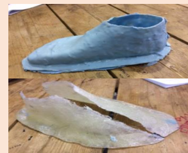
The mold of SACH foot using silicone and fiberglass
