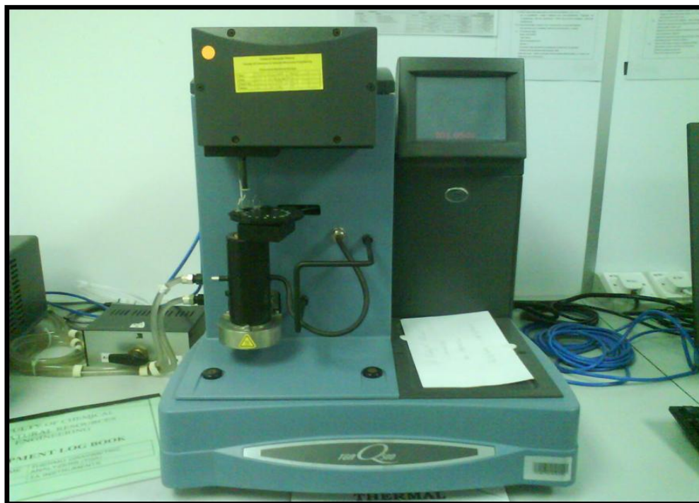
Figure 3.1: TGA (Thermal gravimetric analysis) Q500
