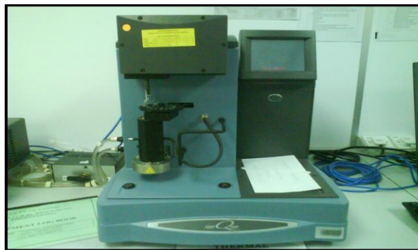
Figure 3.1: TGA (Thermal gravimetric analysis) Q500
