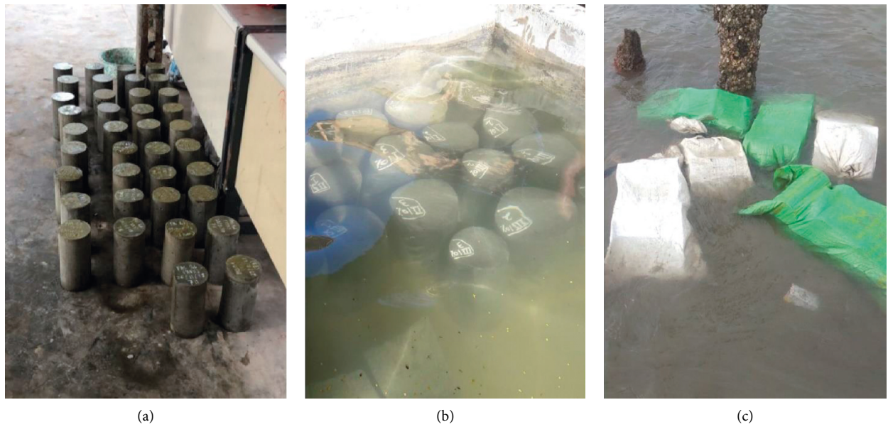
FIGURE 4: Sample preparation: (a) sample after 24 hours casting, (b) sample in distilled water immersion, and (c) sample in sea water immersion.
