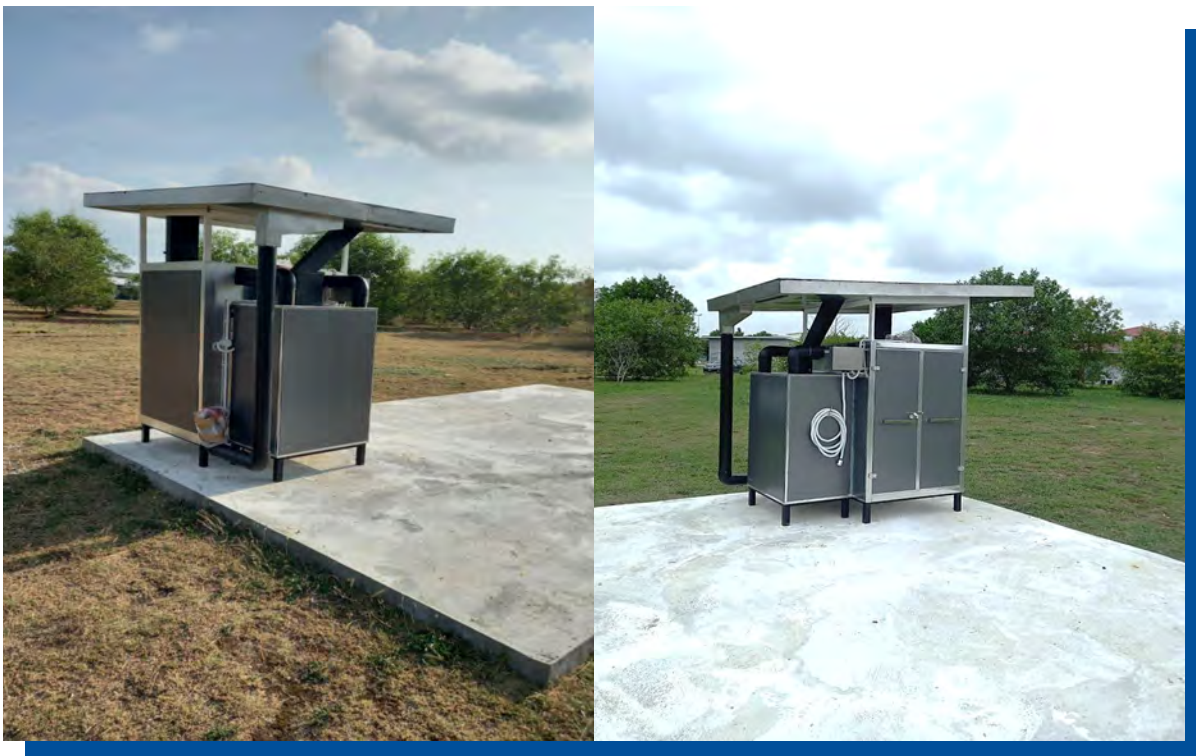
Figure 3. Hybrid solar-heat pump dryer developed at UMP
