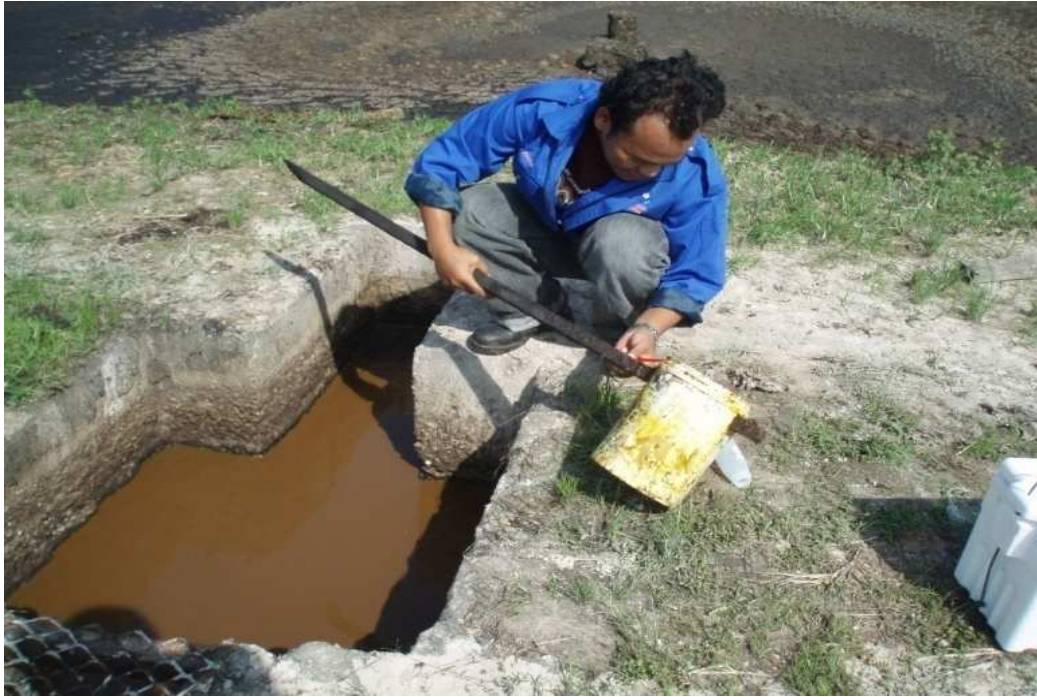
Figure 4.4: Oil carryover to anaerobic pond 1
