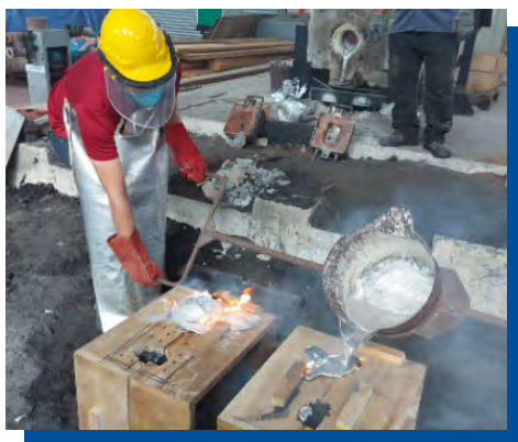
Figure 9. Molten metal pouring process
