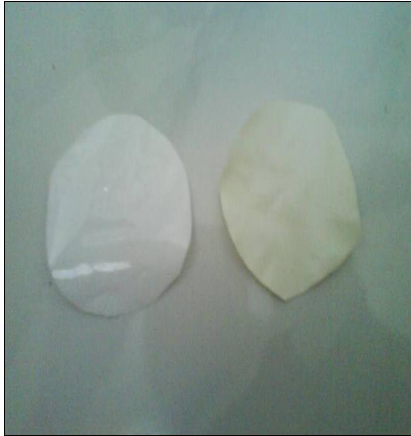
Figure D: Sample of membrane uncoated and coated with bromine
