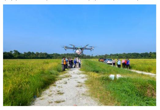
"It can be controlled at a distance with a height of 30 meters and with a maximum speed of 10 meters per second.
