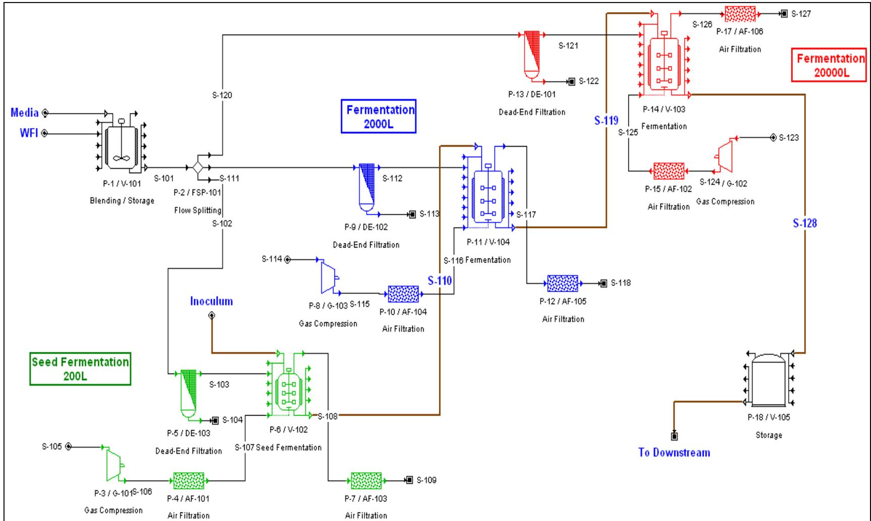
Figure 4.2: Flow work for upstream process
