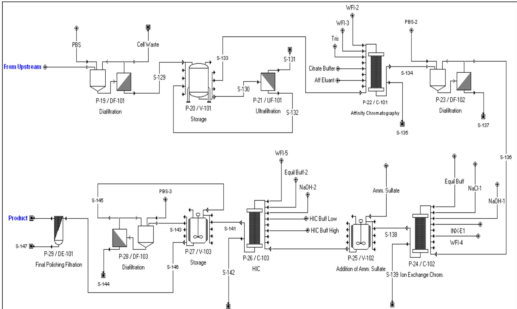
Figure 4.3: Downstream process for SPD source
