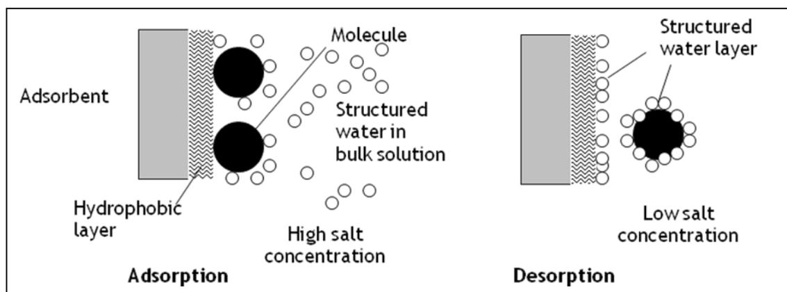
Figure 2.7: Hydrophobic interaction based adsorption (R. Ghosh, 2006).
