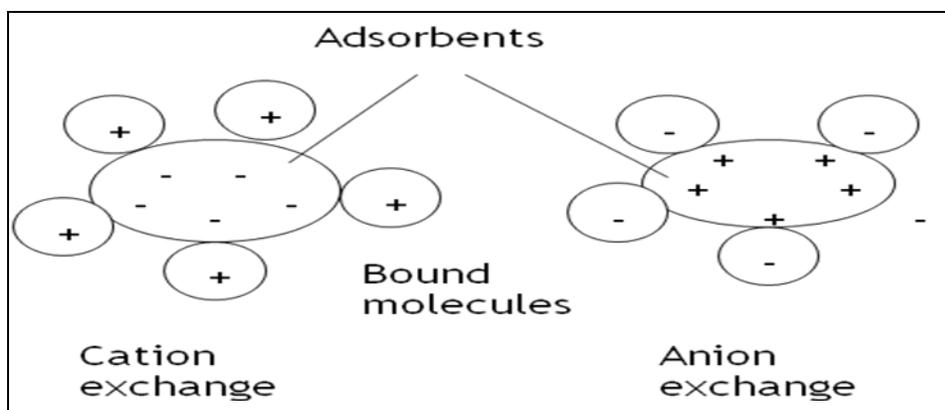
Figure 2.6: Ion exchange based adsorption (R. Ghosh, 2006).
