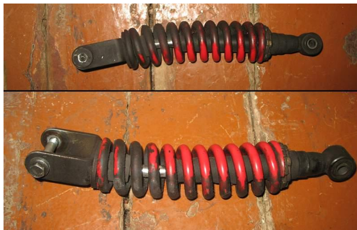
Figure 3.8: Bending damper problem.
