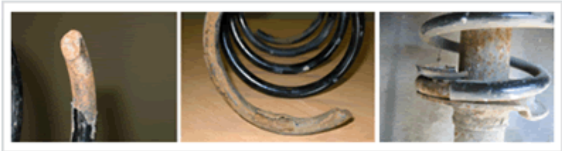
Figure 3.10: Corrosion at spring.
