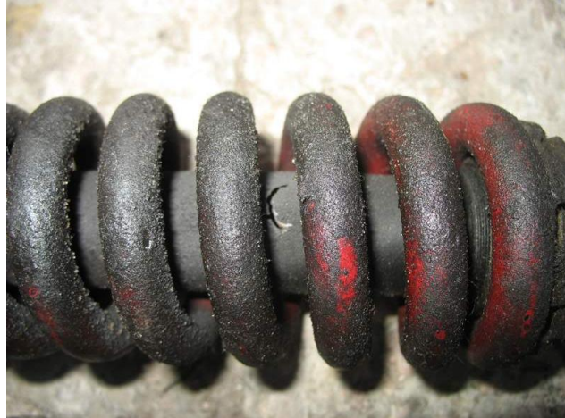
Figure 3.7: Crack at damper cylinder.
