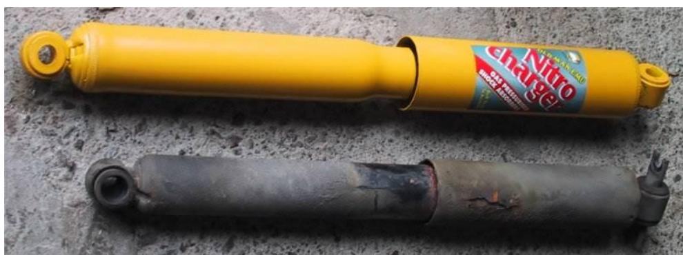
Figure 3.6: Comparison between good damper and broken damper.
