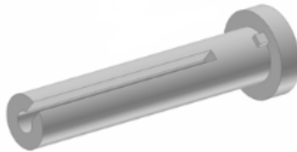
Figure 2.8: Plunger design of IKV machine
