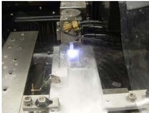
Figure 3.11: Electrical Discharge Machine process
