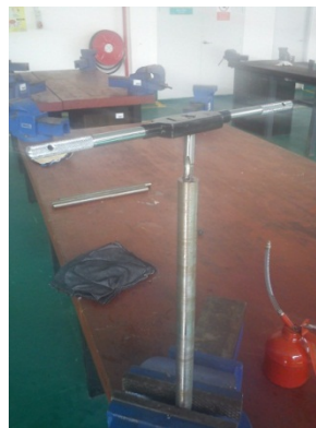
Figure 3.9: Threading process in the hole
