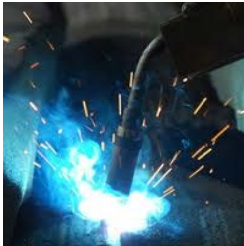
Figure 3.10: Welding process by MIG welding machine
