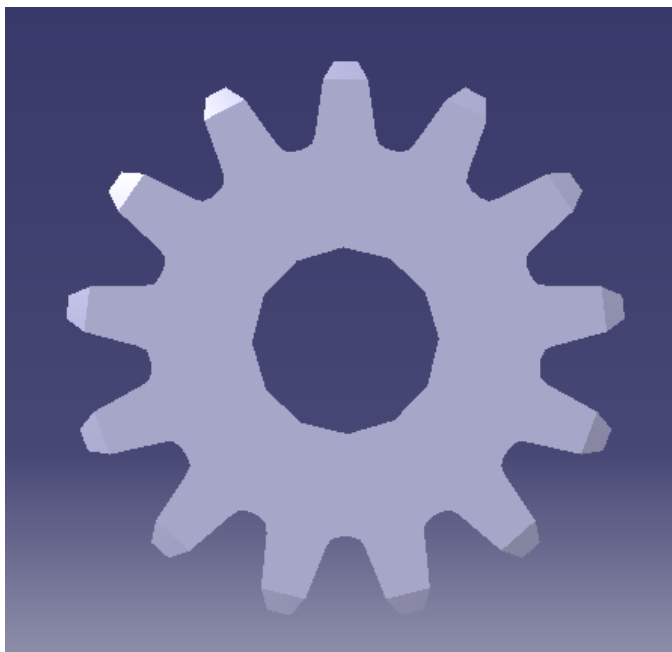
Figure 4.5: Side view of spur gear
