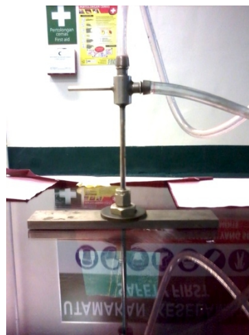
Figure 3.6: Connection of Clear Tube to Pitot Tube
