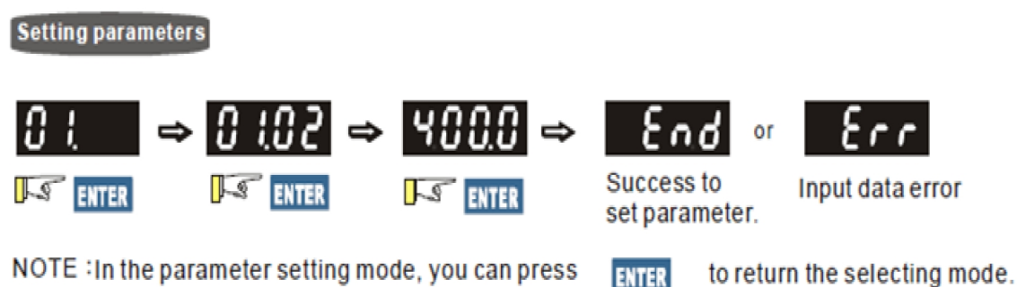
Figure 3.3: Procedures to Set the Parameter of AC Inverter
