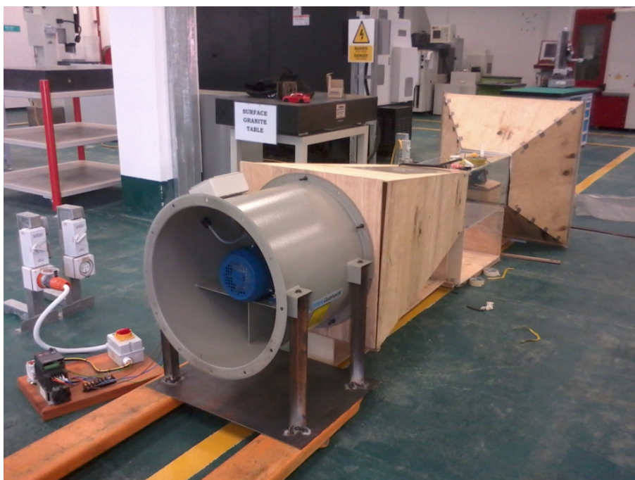
Figure 4.2: Attachment of Fan System to Wind Tunnel
