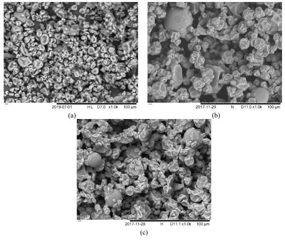
Fig. 4: SEM micrographs of powdered samples obtained at (a) without maltodextrin DE 10 and feed flow rate of 2115 ml/h, (b) with maltodextrin DE 10 and feed flow rate of 2115 ml/h, and (c) with maltodextrin DE 10 and feed flow rate of 485 ml/h. The inlet dry air temperature and air flow rate were fixed at 200 °C and 3.5 m/s, respectively.
