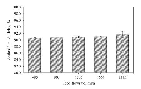
Fig. 2: Antioxidant activity of spray dried powder at different feed flow rates with 0.40 average standard deviation.
