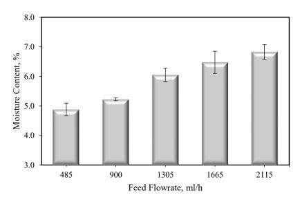
Fig. 1: Moisture content of spray dried powder at different feed flow rates with 0.224 average standard deviation.
