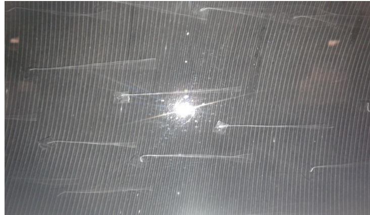
Figure 4.6: Strings show turbulent flow in test section at air speed of 58 m/s
