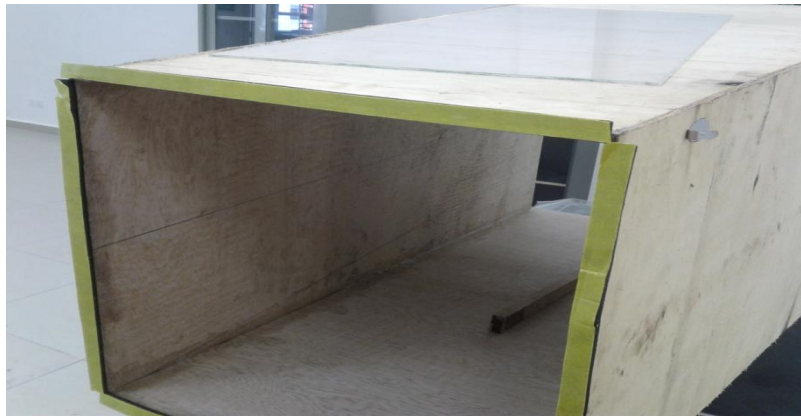
Figure 3.7: Installation of rubber gasket
