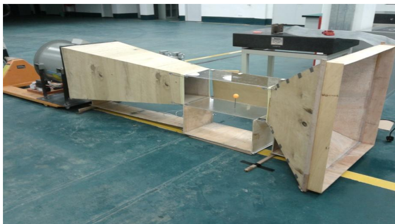
Figure 3.8: Complete assemble of wind tunnel
