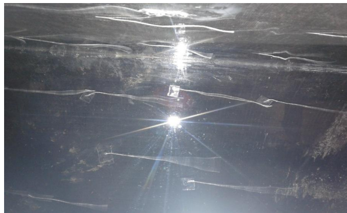
Figure 4.5: Strings show tuberlent flow in test section at air speed of 23 m/s
