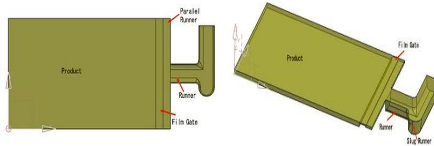
**Figure 2.2:** Film gate with main parts
