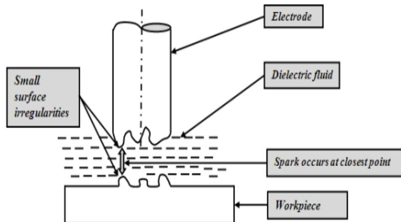
**Figure 2.3:** Working principle of EDM
