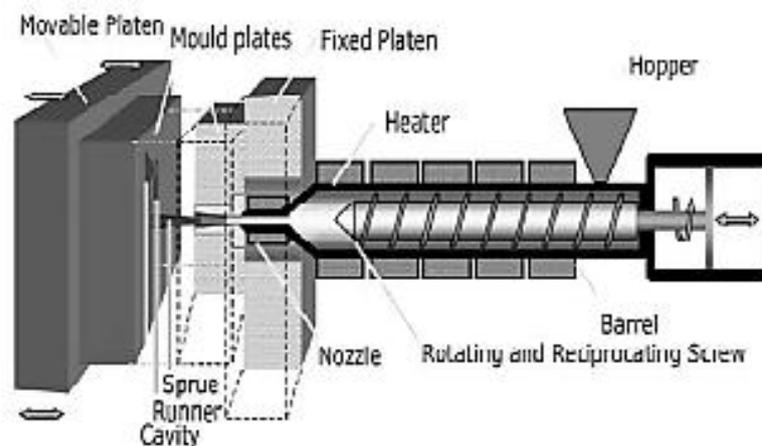
**Figure 2.4:** Injection molding machine with reciprocating screw
