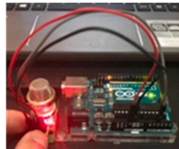
Fig. 8. Calibration of MQ 136 sensor for SO 2 .
