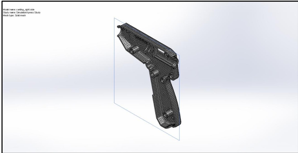
Figure 4.13: Mesh of Canting tool body
