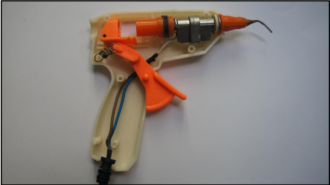
Figure 2.24: Inside view of canting tool
