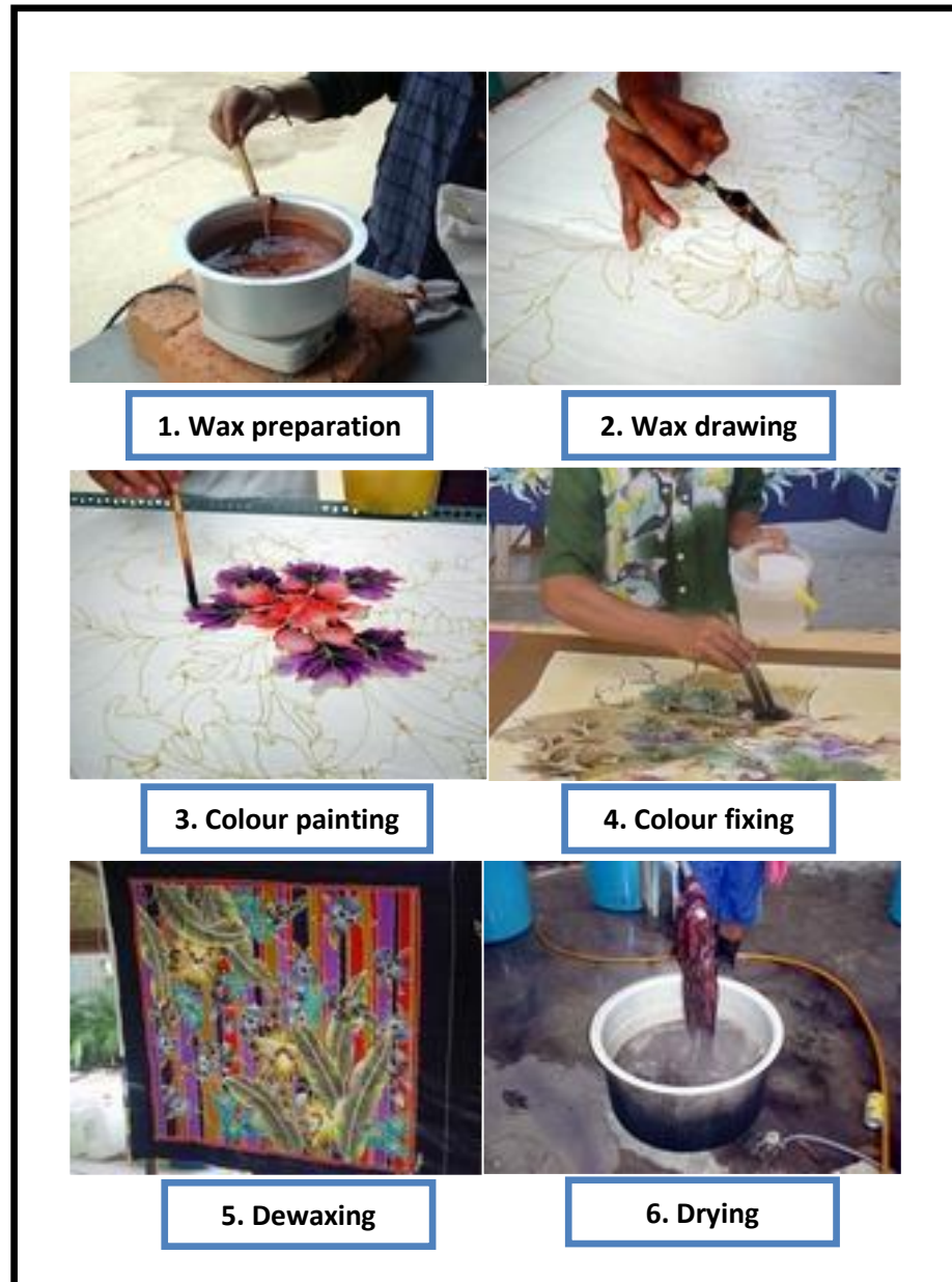
Figure 2.1: Traditional Process of Making Batik
