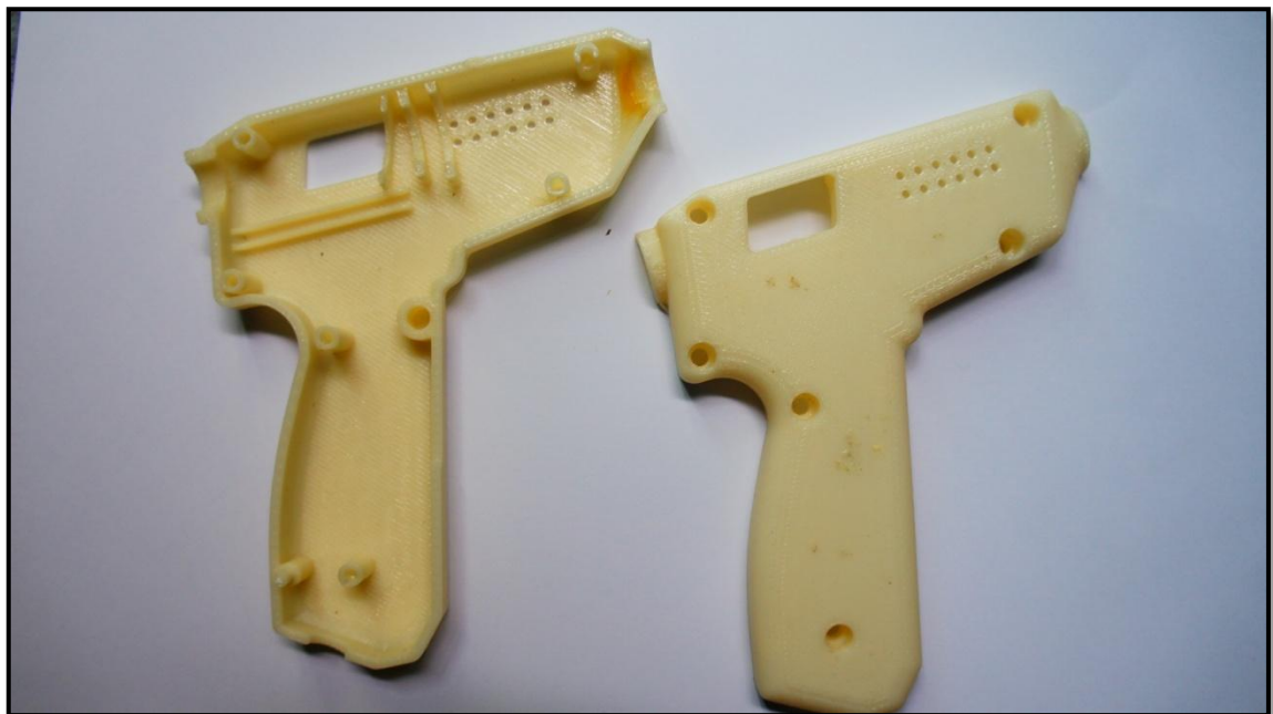
Figure 4.22: Prototyping of the canting body
