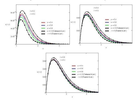
**Figure 6.** Velocity profiles u(r, t) versus *r* for different values of the fractional parameter  $\alpha$ .
