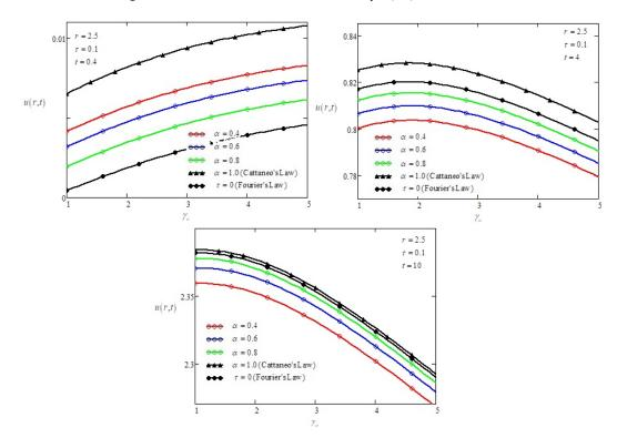
**Figure 8.** The variation of the fluid velocity with the Casson parameter  $\gamma_0$ .
