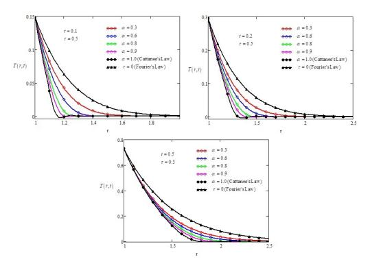
**Figure 2.** The profiles of the nondimensional temperature T(r, t) for different values of the fractional parameter.
