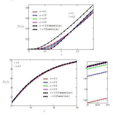
**Figure 3.** Time-variation of the nondimensional temperature T(r, t) for different values of the fractional parameter.
