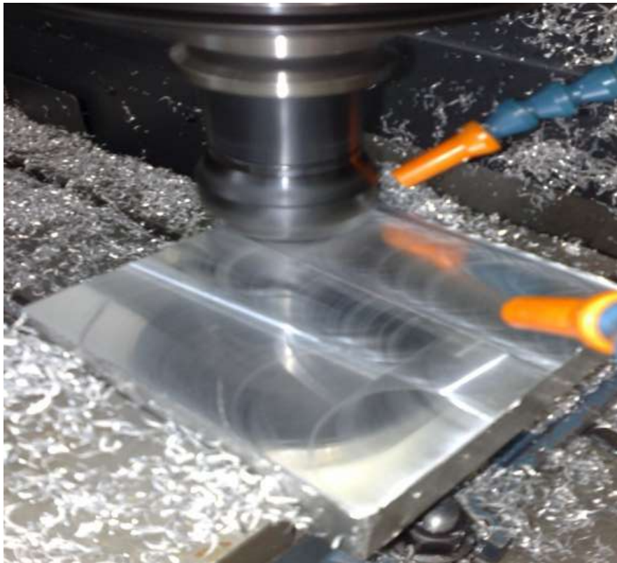
Figure 4. 3 : Machining the Mould
