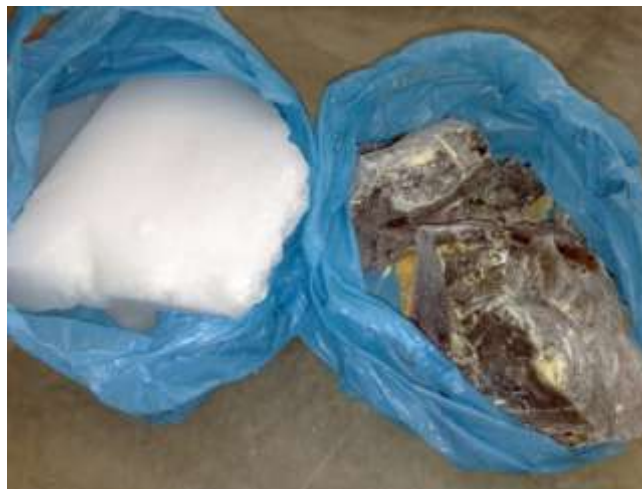
Figure 3.2 : Raw material of (1) Paraffin (2) Resin (Dammar Gum)
