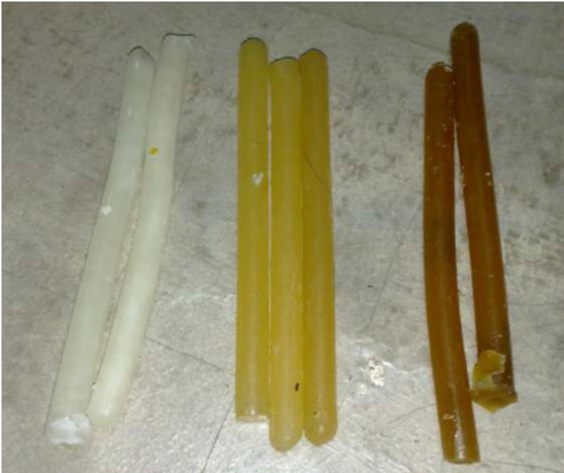
Figure 4. 7 : (1) 65% of paraffin and 45% of resin (2) 50% of paraffin and 50% of resin (3) 45% of paraffin and 65% of resin
