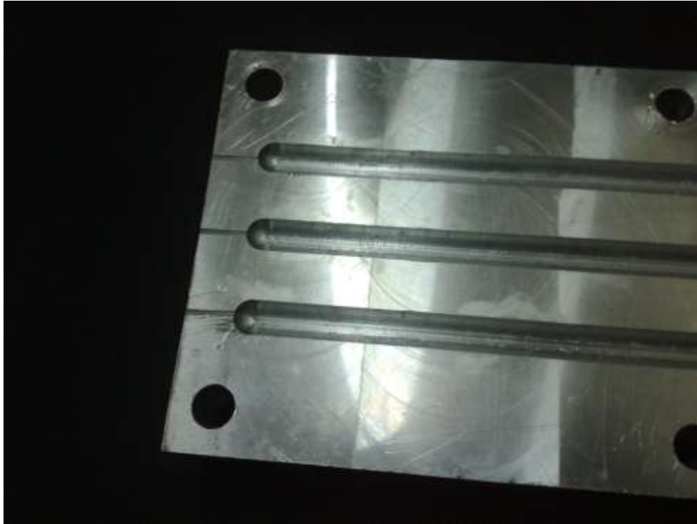
Figure 4. 5 : Air Vents at the end of the cavity slot
