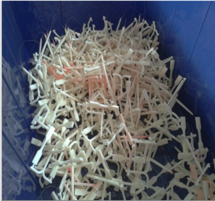
Figure 3.2: Abs products with runner and sprue
