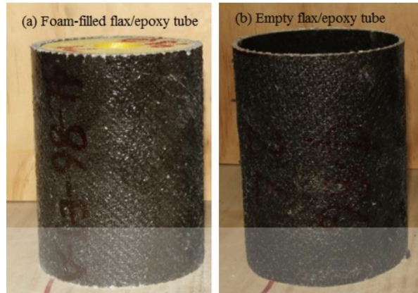
Figure 2.9 (a) Foam-filled flax/epoxy tube (b) empty flax/epoxy tube Source : Yan et al., (2014b)
