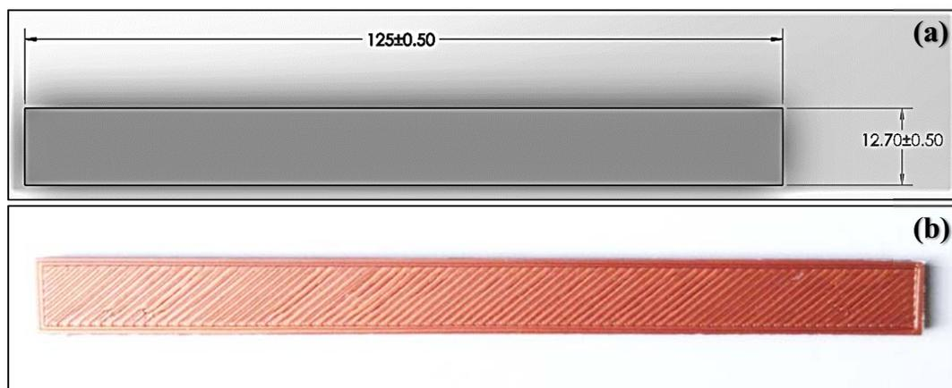
**Figure 3.** (a) Dimension of the test specimen, (b) 80 wt.% Cu with Concentric infill pattern flexural test specimen, (c) 25 wt.% Cu with Rectilinear infill pattern.
