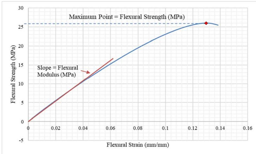
**Figure 4.** Stress vs strain curve of a sample specimen with Octagram-spiral infill pattern and 25 wt.% Cu composition.
