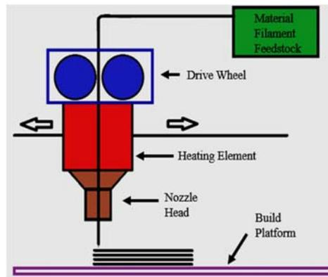
**Figure 1.** Fused deposition modelling working mechanism.
