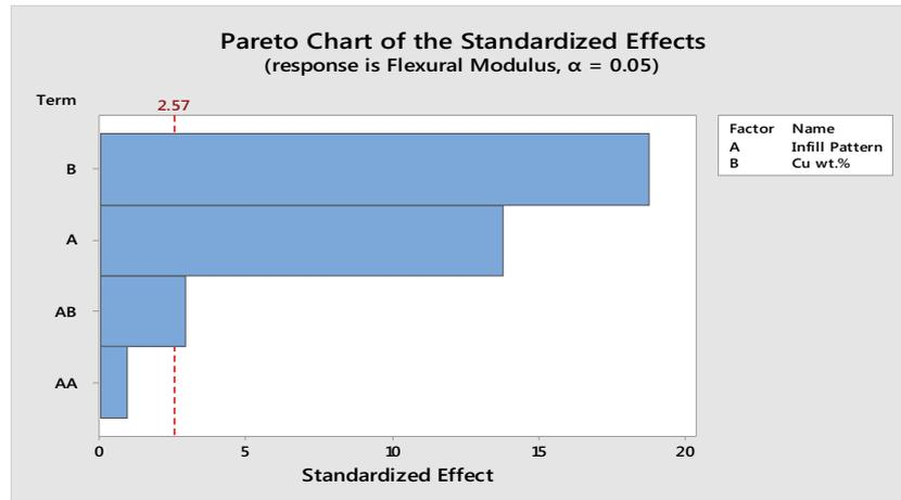
Figure 8. Pareto chart of printing parameters toward flexural modulus.
