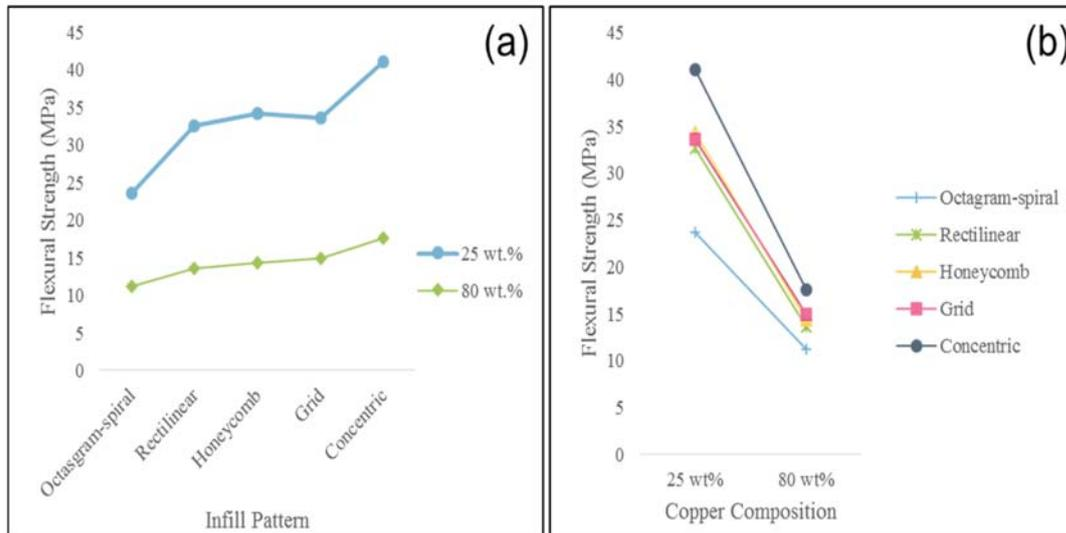
Figure 5. Graph of flexural strength against infill pattern and copper composition.
