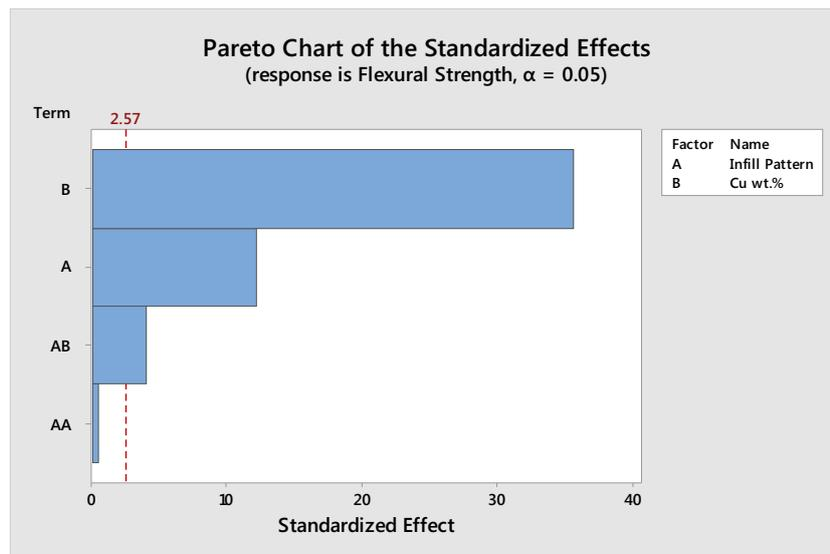
Figure 6. Pareto chart of printing parameters toward flexural strength.
