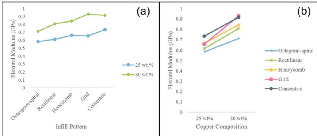
Figure 7. Graph of flexural modulus against infill pattern and Copper composition.
