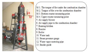
Fig. 1 Schematic Diagram for FBC
