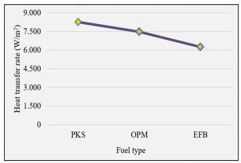
**Fig. 4** Heat transfer rate for different fuel
