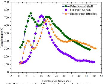
Fig. 9 Temperature for different fuel and combustion time
