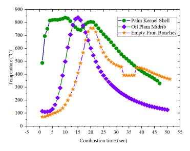
Fig. 7 Level of temperature for different fuel and combustion times (9)
