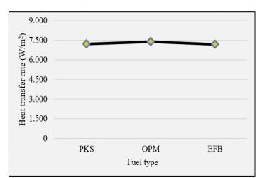
Fig. 6 Heat transfer rate for different fuel
