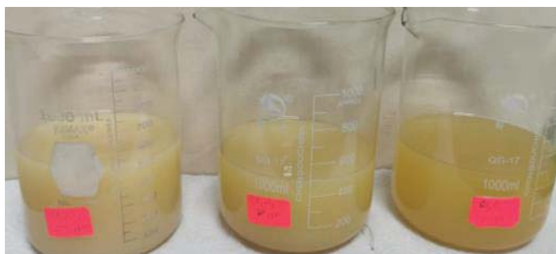
FIGURE 3. Df+( Ce_2O_3 ) nanoparticles in concentrations 25, 50, and 75 ppm from right to left accordingly.
