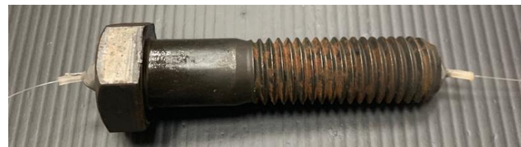
Embedded FBG smart bolt
