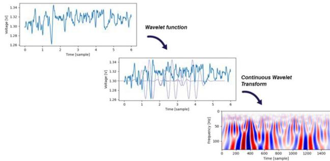
Fig. 1. Process of CWT.
