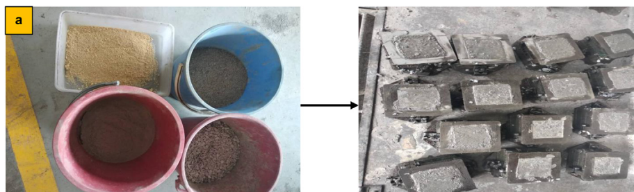
Fig. 6. Preparation of raw materials: (a) raw materials for mixing concrete, (b) materials after mixing and putting in the cube.
