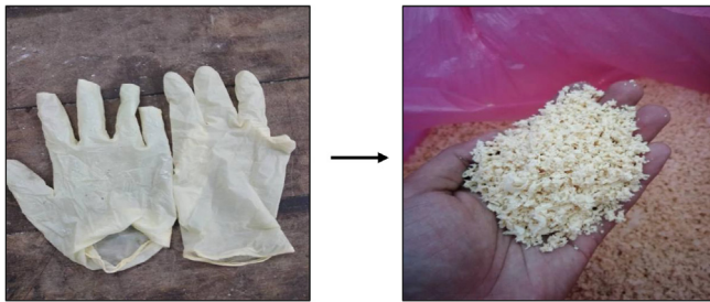
Fig. 4. Latex glove (LG) waste before and after shredding to size 1–5 mm.
