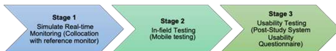
Figure 1. Proposed three-stage framework for evaluation of wireless outdoor individual exposure indicator system
