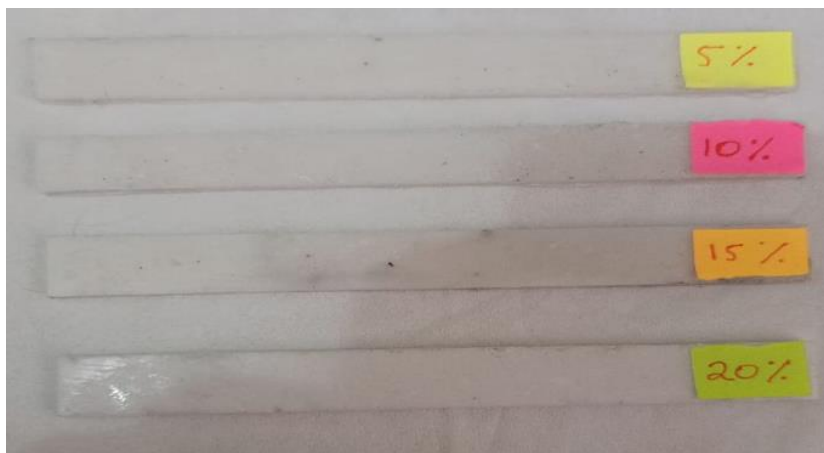
Figure 3. Biocomposite Specimens Produced with Variations of HA
