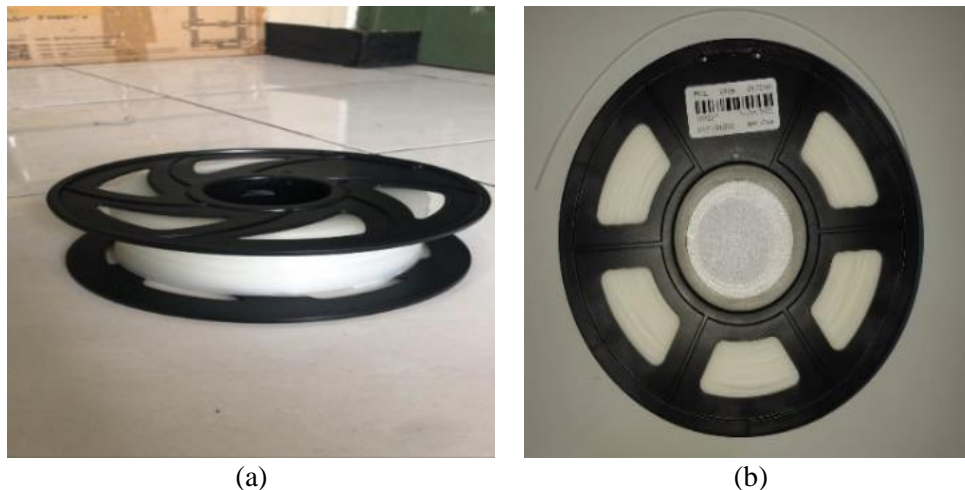
Figure 1. Filament (a) Polylactid Acid (PLA) (b) Polycaprolacton (PCL)
