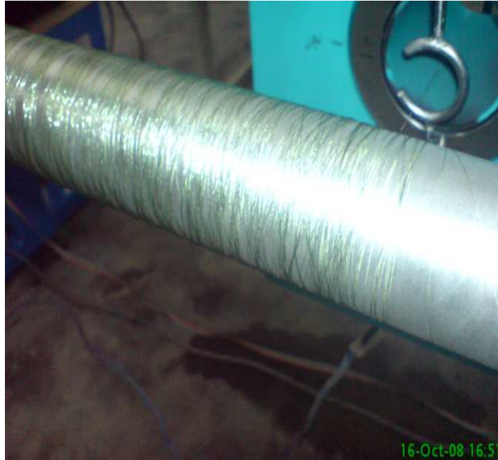
Figure 5.7 the fiber half covered the mandrel
