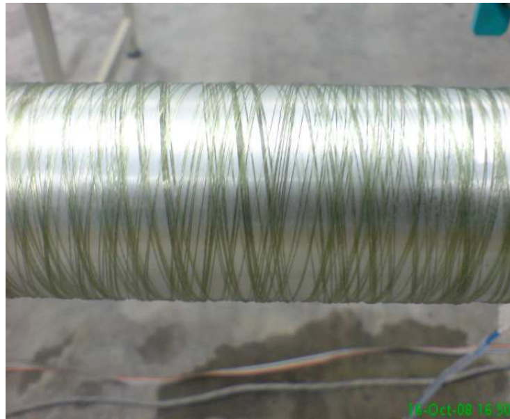
Figure 5.6 the dry fiber covered the mandrel
